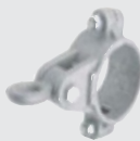
REGULAR BEARING HANGER Galvanized ductile iron. Comes with oil-infused bronze bushings. SP-14 89mm (3-1/2") beam SP-15 60mm (2-3/8") beam
