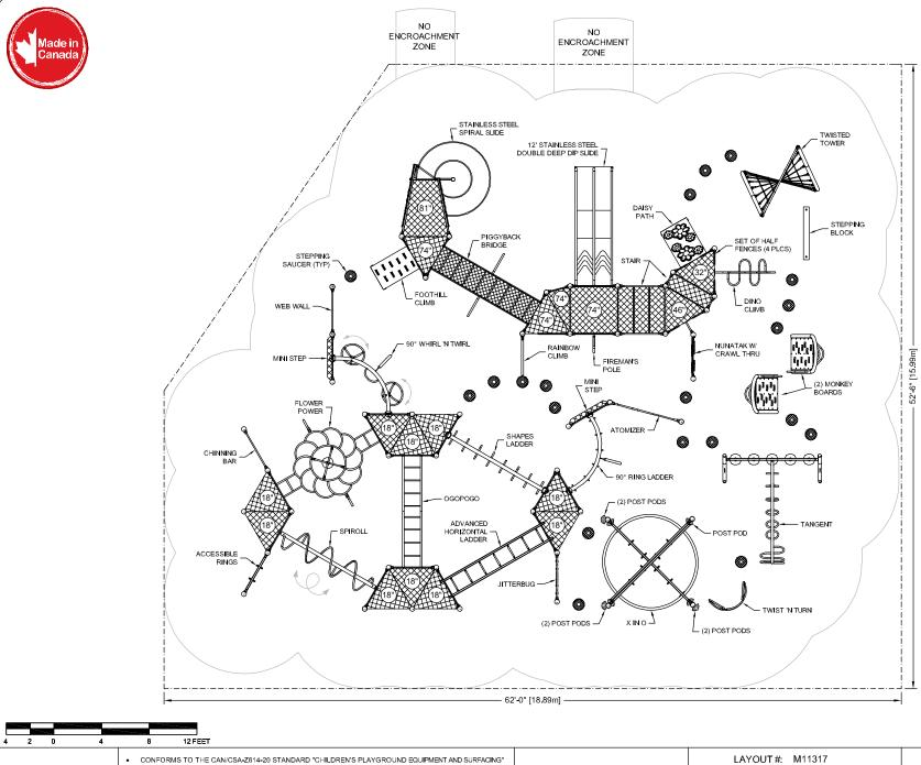
PERIMETER SHOWN REPRESENTS EXTENT OF REQUIRED SAFETY SURFACING, WIDTH OF BORDER MATERIAL MUST BE ADDED BEFORE EXCAVATION.
