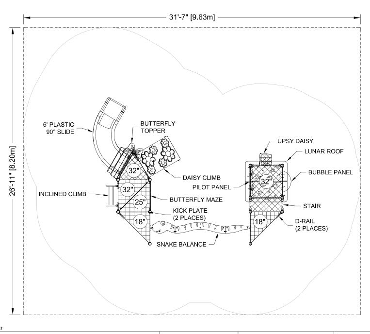
BLUE IMP SLIDES MUST BE INSTALLED WITH SLIDE BEDS FACING BETWEEN NORTH AND EAST CONFORMS TO THE CAN/CSA-Z614-20 STANDARD "CHILDREN'S PLAYGROUND EQUIPMENT AND SURFACING"
