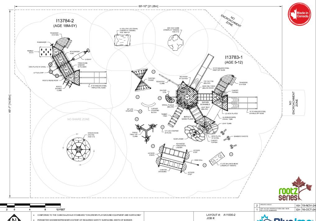
BLUE IMP SLIDES MUST BE INSTALLED WITH SLIDE BEDS FACING BETWEEN NORTH AND EAST
