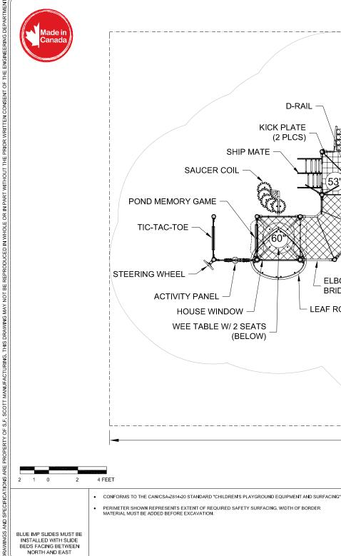
PERIMETER SHOWN REPRESENTS EXTENT OF REQUIRED SAFETY SURFACING, WIDTH OF BORDER MATERIAL MUST BE ADDED BEFORE EXCAVATION.
